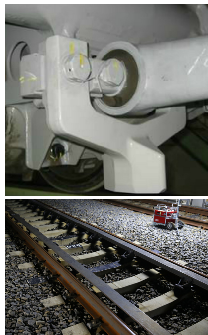
Image of vehicle (top) and lane deviation prevention device (Courtesy of JR Central)
