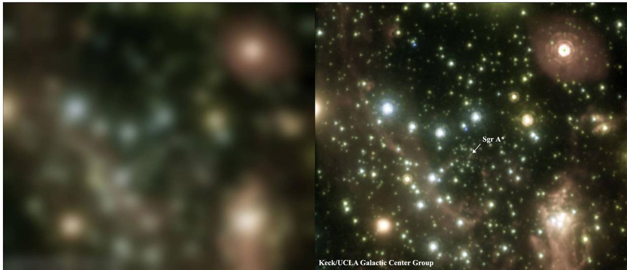
**Image 2:** Comparison of simulation images of the galactic center by the Subaru Telescope (left) and TMT (right). A very sharp image is obtained after correcting the influence of Earth's atmosphere with adaptive optics technology. The large diameter TMT can achieve four times as high or greater resolution than the Subaru Telescope. (Photos: Keck/UCLA)
